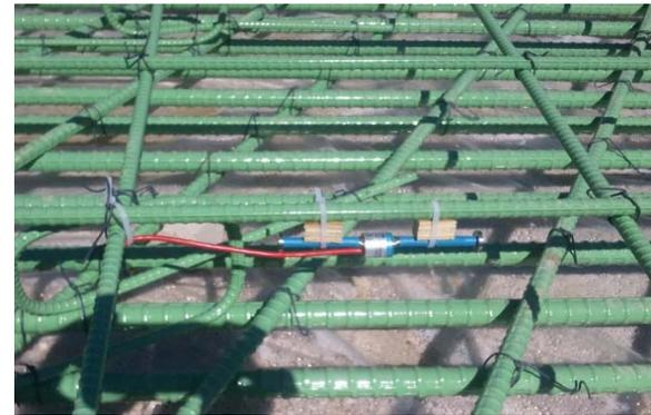
*Approach slab embedded strain gage instrumentation*
