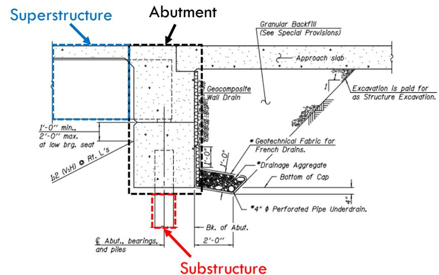
Typical Integral Abutment Detail (IDOT Bridge Manual, 2012)
