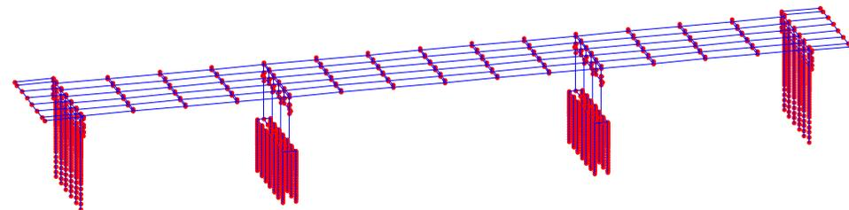
Schematic of the three-span IAB used for modeling in OpenSees
