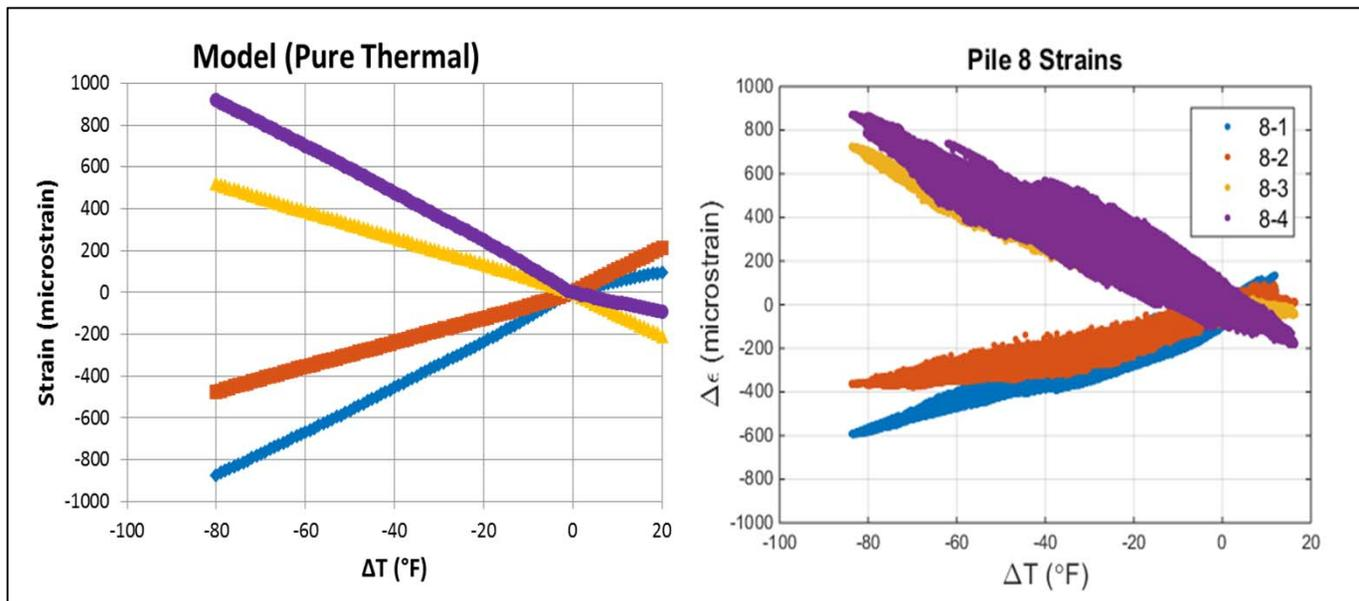
Axial contribution causes upward shift in magnitude; strong-axis bending causes a separation between gage pairs
