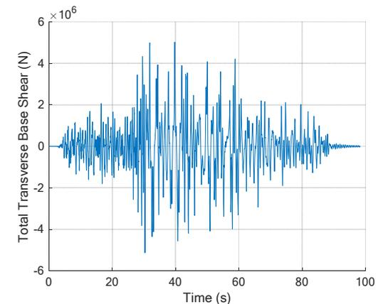
Total base shear in a three-span steel IAB during a ground motion
