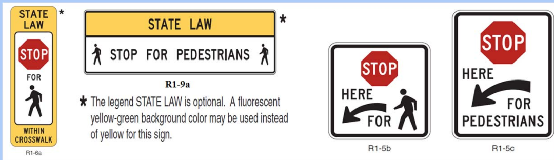
Uncontrolled pedestrian crosswalk signs
