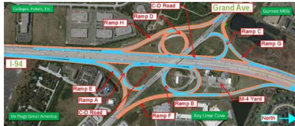
Improved Full Cloverleaf with Collector-Distributor Lanes
