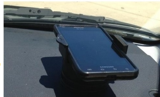
(a) Cellphone App Capturing Vertical Acceleration
