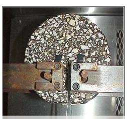
**DCT (ASTM D7313)**
