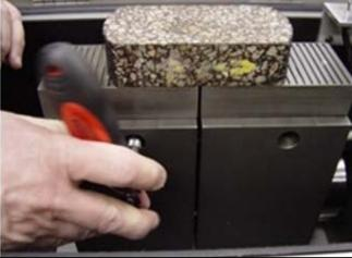
**DCT (ASTM D7313)**
