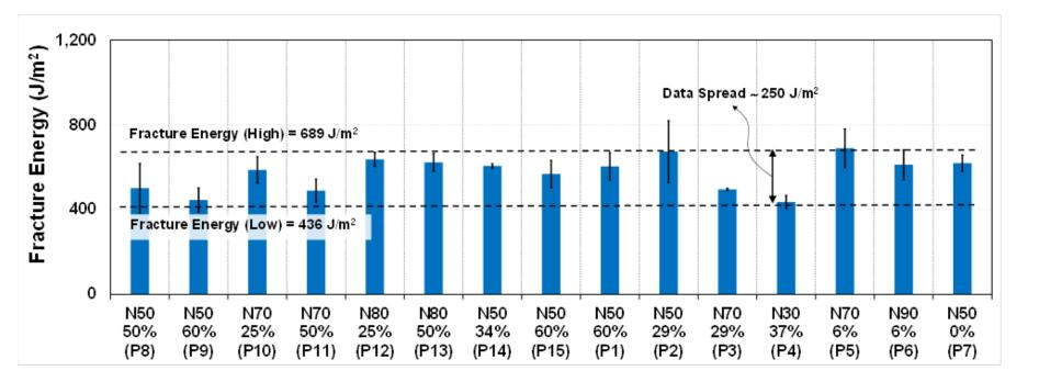
SCB fracture test results at -12°C
