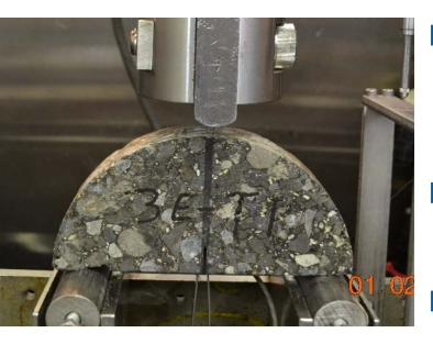
**Relies on** simple three point bending Easy specimen preparation □ Can use **AASHTO T283** equipment \* **Repeatable**
