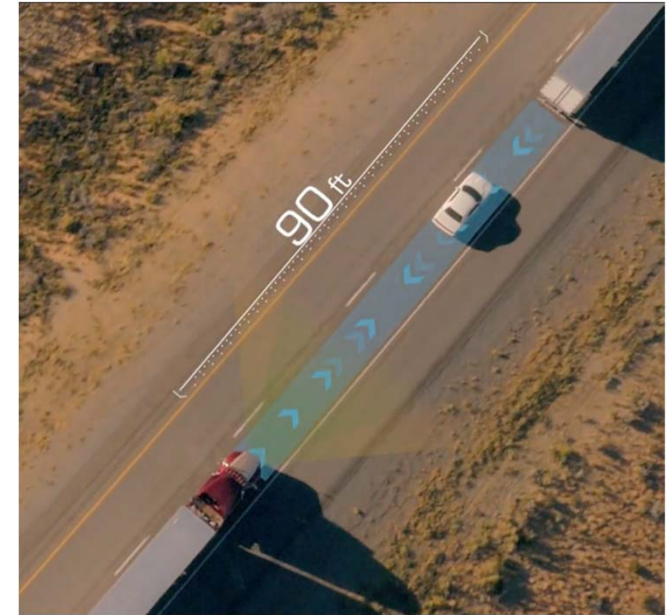
Follow truck will continue to back off to safe manual following distance (100+ ft) and then give full manual control back to follow driver
